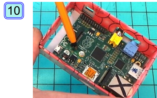
Bolt Raspberry Pi in the Case4-Pi (the pen points to the 'nut and bolt' position)
